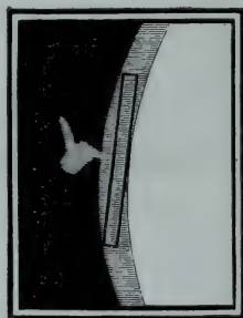
SLIT PLACED TANGENTIALLY TO VIEW A PROMINENCE.
